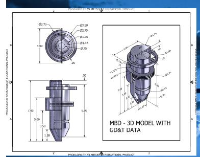
The electronic elements that specify the 3D Computer Aided Design (CAD) geometry and all design requirements for a product (including notations and parts lists), and the use of this data throughout an integrated CAD Systems, typically consisting of; Computer Aided Manufacturing (CAM); Coordinate Measurement Systems (CMS) and use of Coordinate Measurement Machines (CMM)
